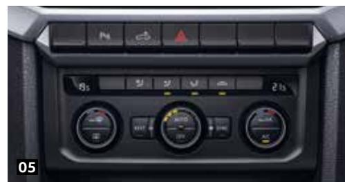
**05 "Climatronic" air conditioning.** This system offers 2-zone temperature control for the driver and front passenger. Depending on the intensity of the sun's rays and the outside temperature, the air conditioning adds more or less cool air accordingly. | SL | HL | UL |
