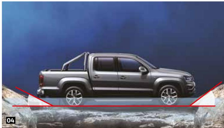
**01 Side slope angle.** The broad track of the Amarok provides enormous stability even when driving along slopes with up to a 50° incline.<sup>1)</sup>
